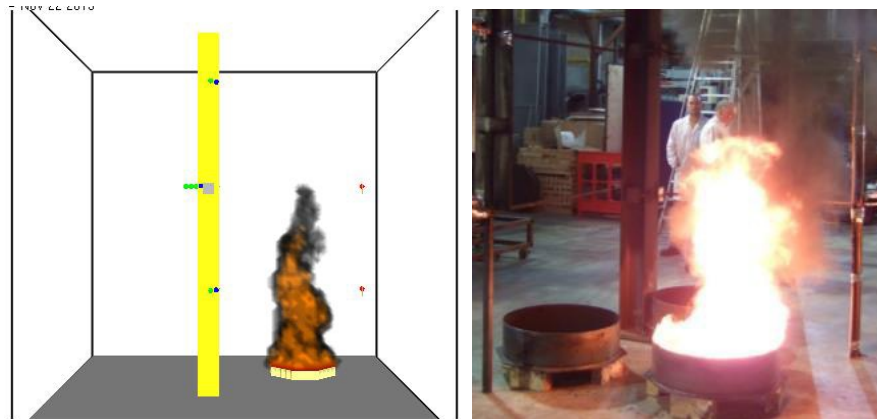
Figure 3.6 Comparison between flame shape prediction by FDS and a photograph of the test, for FireSERT test Column I2 - I11 [17]
