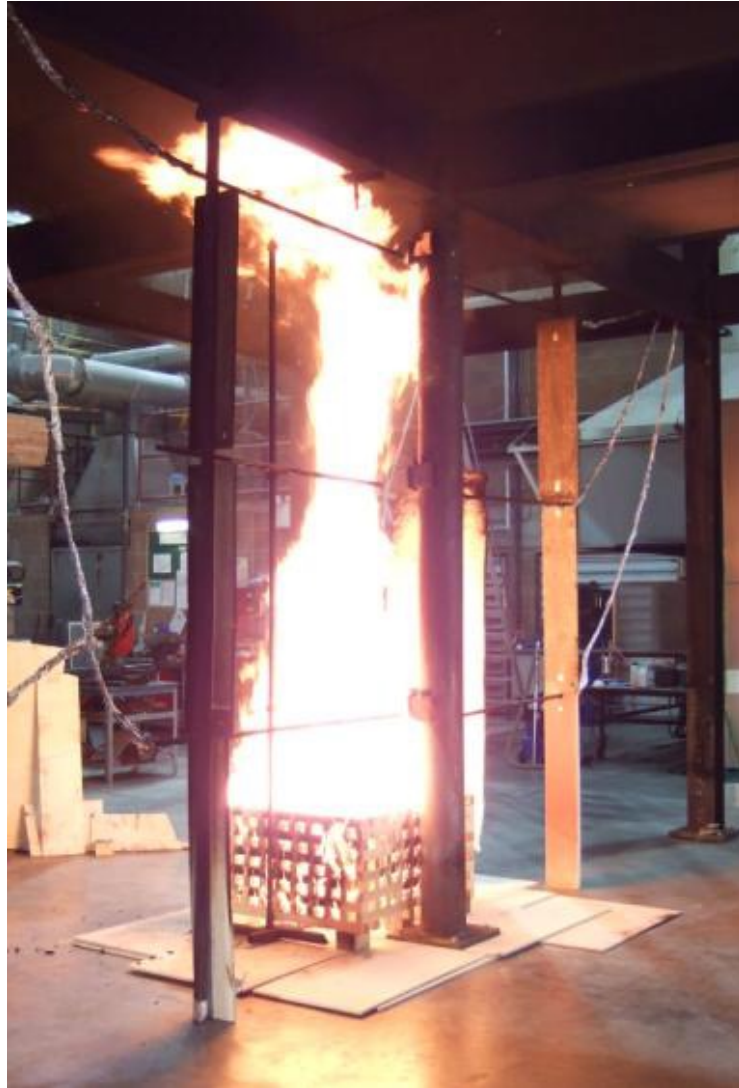
Figure 3.5 Fire impacting the ceiling
