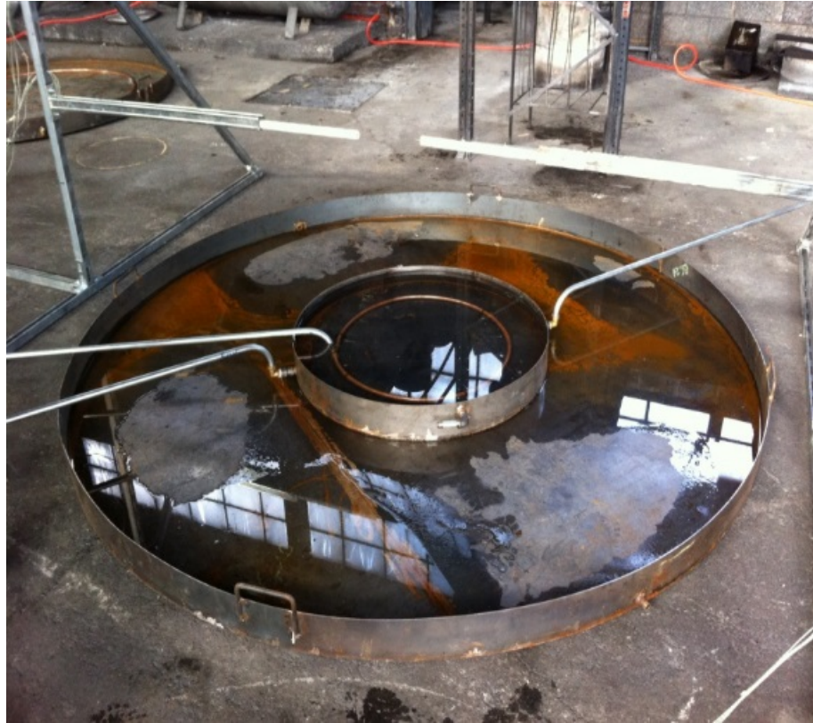
Figure 3.3 2 m test pan, showing fuel feed mechanism (from LOCAFI Deliverable 15 [13] )
