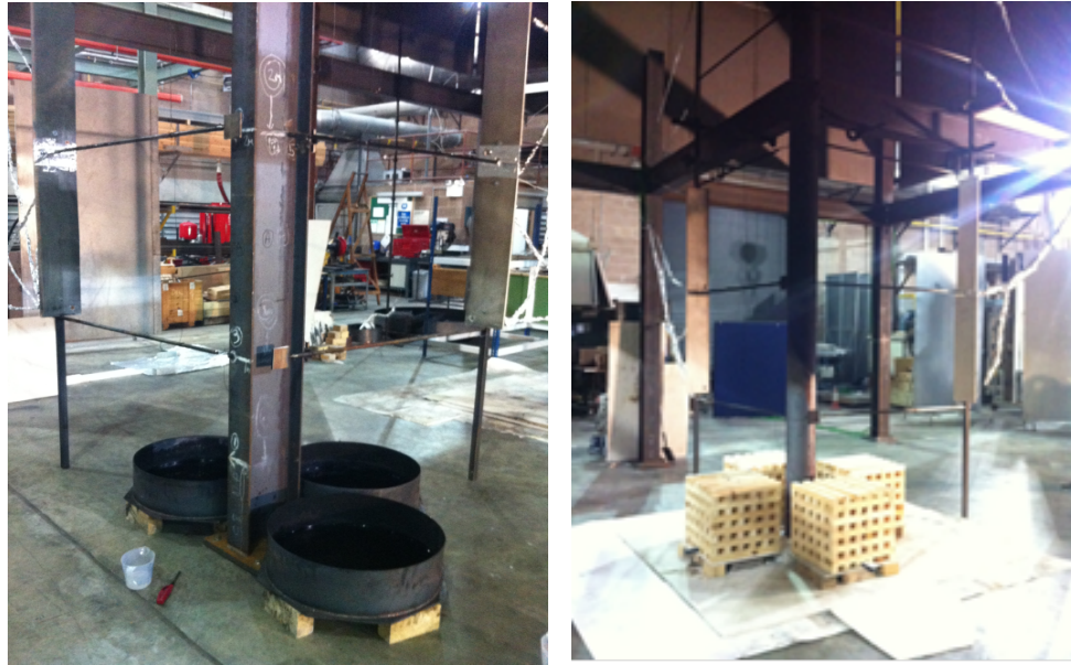
Figure 3.4 Test set-up for localised fire tests at FireSERT (left: basins for containing liquid fuel, right: wooden cribs) [15]
