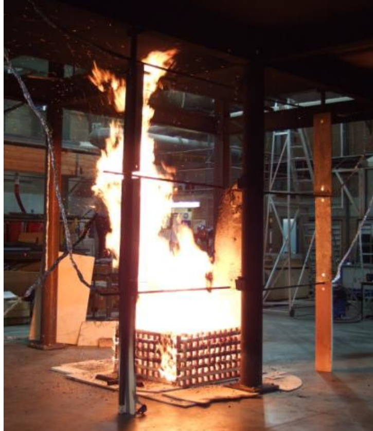
Figure 3.7 Test O36, showing flame tilting [15]
